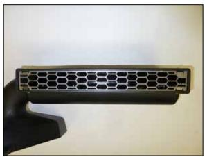
9. Install the inlet mesh into the K&N<sup>®</sup> fresh air intake and secure with the provided hardware.
