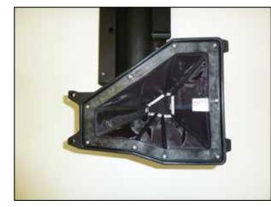
7. Install the dry charger assembly into the K&N<sup>®</sup> fresh air intake system and secure with the provided hardware.
